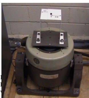
Figure 2 showing component attached to VP30 Vibrator prior to testing
